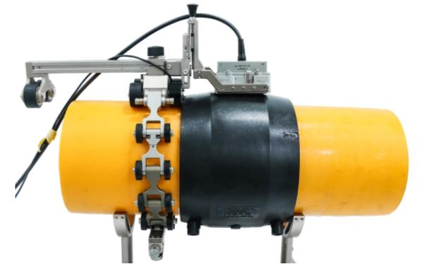
PE管电熔对接接头检测
